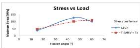
a) Cocr and Ti6Al4V+Ta
