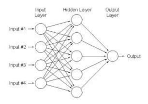
Fig.2. Multilayered Neural Network
